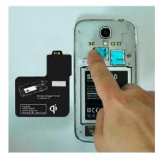
**4)** Replace back cover. Phone is now ready charge wirelessly with any Qi-enabled charger.
