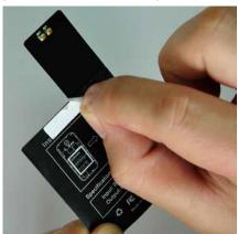
**3)** Align and ensure the receiver pins are in contact with the phone's metal contacts.
